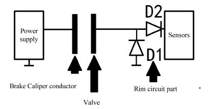
Figure 1 : The principle of indirect TPMS figure
