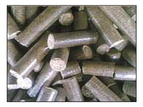
Fig. 1: Briquettes of bio-coal
