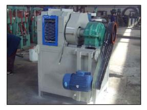
**Fig. 2: Briquetting machine**
