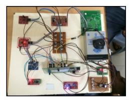
Fig. 2: Hardware circuit of wearable wrist band health monitoring device
