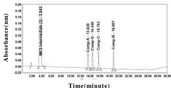
Figure 2: LC chromatogram of montelukast intermediate (2) and its precursors
