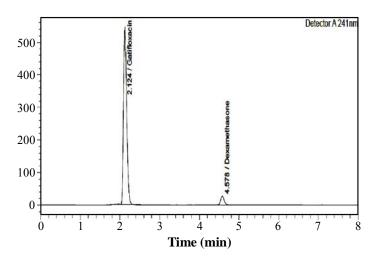
Fig. 4: Chromatogram showing well resolved peaks of GAT and DEX
