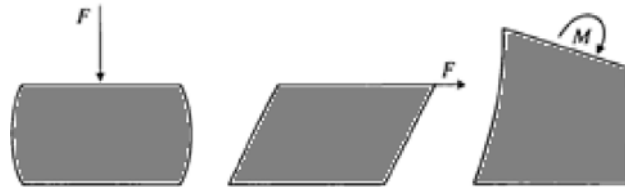
Fig. 1: Principal deformation modes of the rubber block
