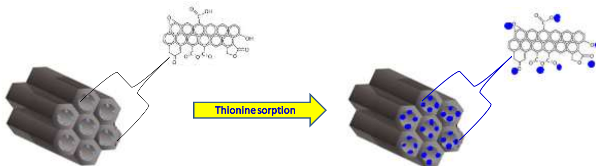
SCHEME.1. Representation of the surface groups and sorption of dye on carbon.
