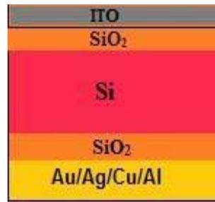
FIG. 3. Multijunction plasmonic solar cell.
