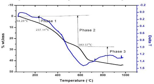
Figure 3 : TGA/DTA results of the purchased OEM friction lining material
