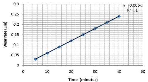
Figure 6 : Time vs. wear for PKS based brake lining
