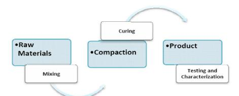
Figure 1 : Flow process for friction-lining formulation and production
