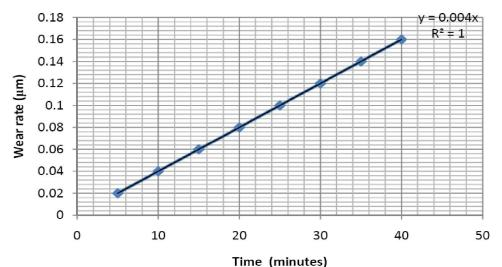
Figure 7 : Time vs. wear for the OEM brake lining
