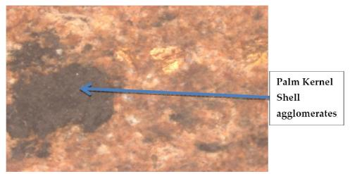
Figure 5 : Optical stereo micrograph of PKS based friction lining produced
