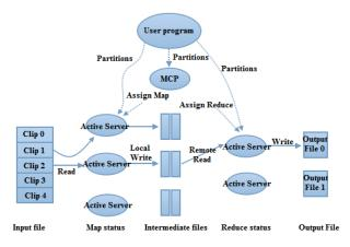
Figure 5: The operation execution process of Map Reduce
