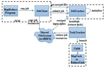
Figure 4 : The principle of how Hadoop operate Map Reduce
