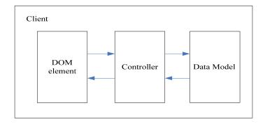
Figure 2: The architecture diagram of client MVC
