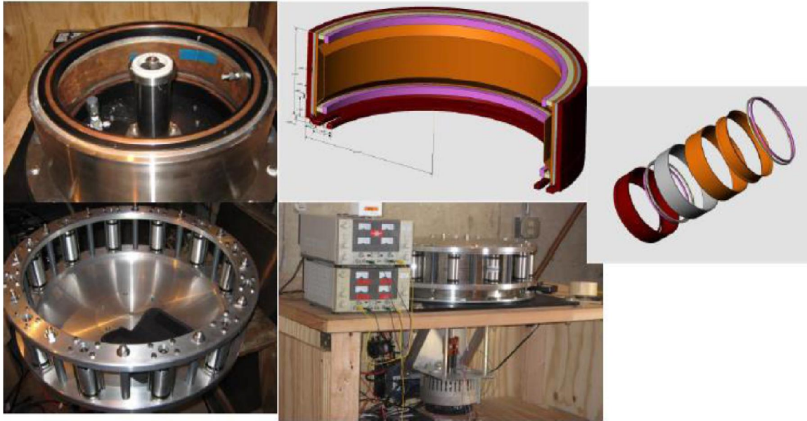
Figure 5 : The laminated ring graphically shows with the actual ring and spindle to drive the carousel. Hardware for the carousel also includes the motor and support drive.
