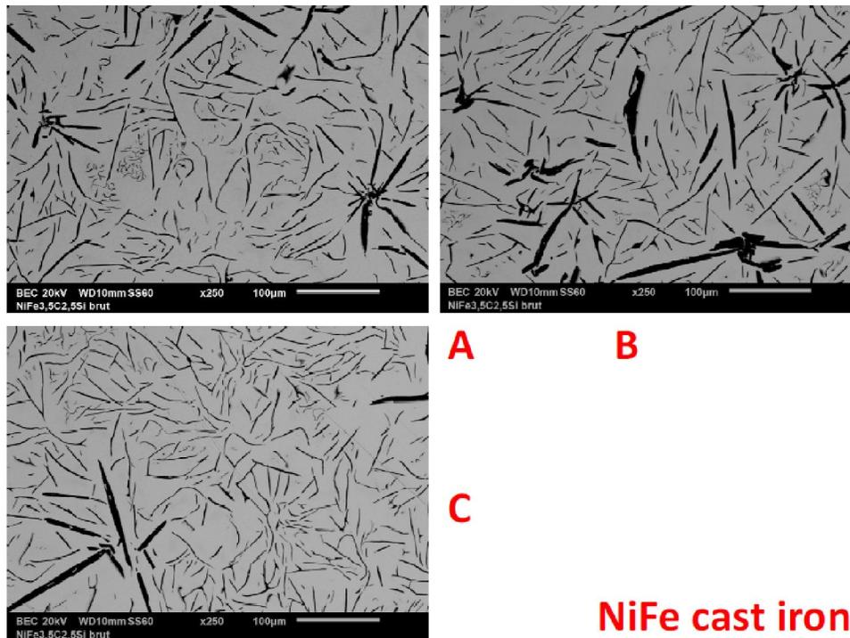
Figure 8 : Microstructure of the “NiFe” cast iron as observed with the SEM (BSE mode) in three distinct zones (“A,” “B” and “C”)
