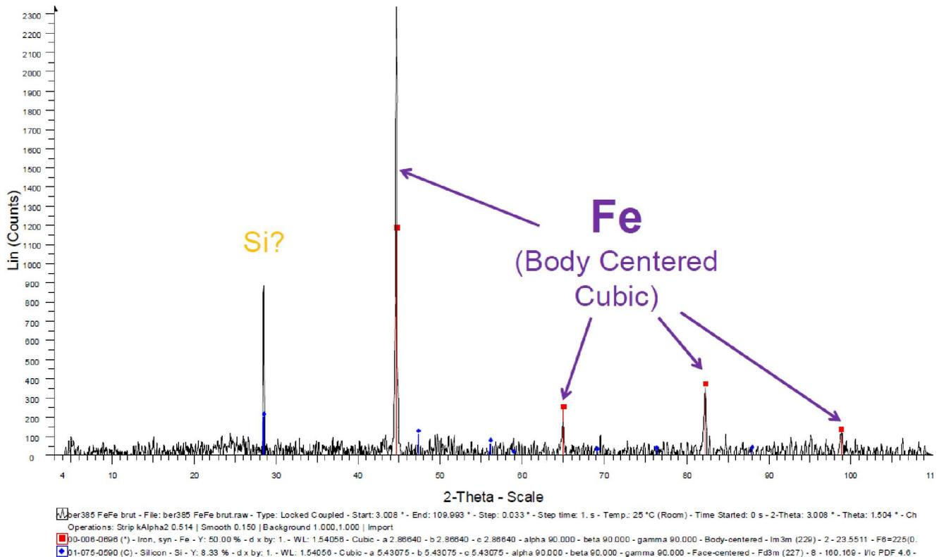
Figure 12 : X-ray diffractogram obtained on the “FeFe” cast iron
