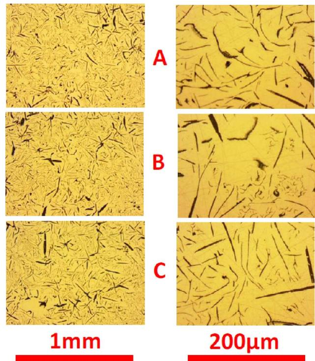
Figure 4 : Matrix structure (after Nital etching) of the "NiFe" cast iron as observed at two magnifications in three distinct zones ("A," "B" and "C")
