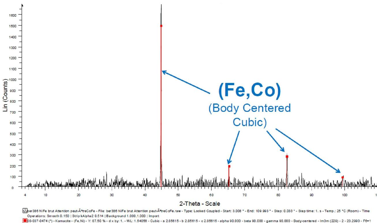
**Figure 10 : X-Ray Diffractogram obtained on the “CoFe” cast iron**
