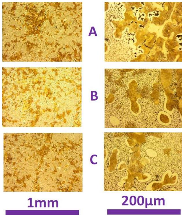
Figure 6 : Matrix structure (after Nital etching) of the “FeFe” cast iron as observed at two magnifications in three distinct zones (“A,” B” and “C”)
