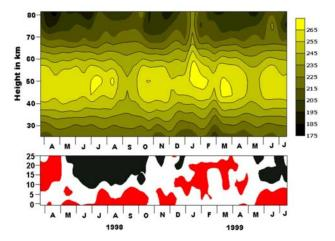
Fig. 3: (top) Time-height contour of lidar temperature from Apr 1998 to Jul 1999; (Bottom) Time-height contour of the radiosonde zonal wind (m/s) westerly winds are ≥ 0 and represented by red colour area; easterly winds are ≤ 0 and represented by black colour area. Contour lines are plotted by steps of 20 m/s
