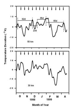
Fig. 7: Deviation from the mean temperature measured at 30 and 50 km. The arrows indicate the dates of the maximum of the 16D wave
