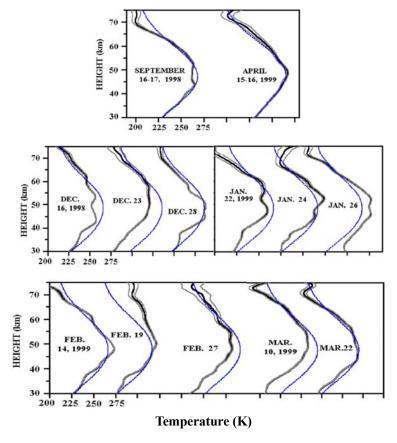
Fig. 1: Series of 13 lidar temperature profiles obtained from Sep.98 to Apr.99. The dotted line represents the MSISE-90 model for the corresponding day and latitude. The standard deviation  $(\pm 1\sigma)$  is indicated
