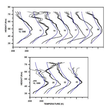
Fig. 4: Lidar temperature profiles for winter Dec. 98-Jan.99 obtained from OHP Rayleigh lidar. T  $\pm$  1 $\sigma$  curves are also shown. The dotted line represents the MSISE-90 model for the corresponding day and latitude
