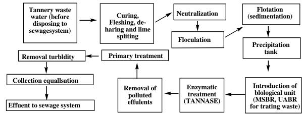
Figure 2 : Schematic diagram for treatment of tannery waste using Biological units and microbial enzymes
