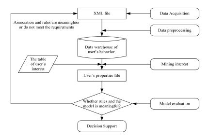
Figure 4: Model of data mining system of users' behavior
