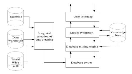
Figure 1 : A typical diagram of data mining system
