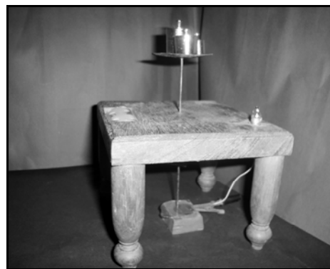
Fig. 2: Instrument for the measurement of hardness of films
