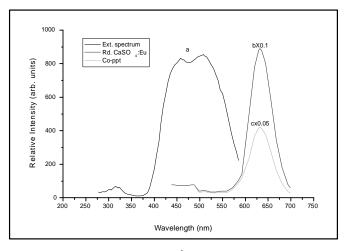
Fig. 1: PL spectrum of CaS : Eu<sup>2+</sup> synthesized by two methods
