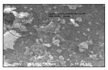
Fig. 2: SEM image of ZnS nanoparticles
