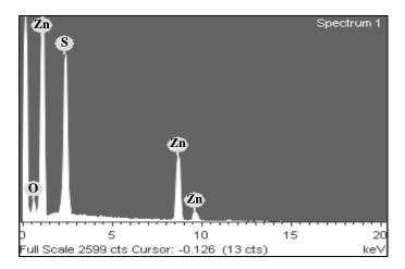
Fig. 3: EDS analysis of ZnS nanoparticles
