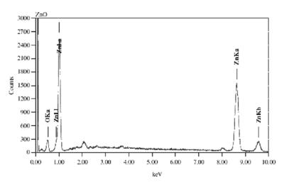
Fig. 4: EDX analysis of ZnO nanoparticles
