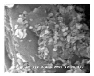
Fig. 6: SEM image of 50% ZnO-Bentonite nanocomposite
