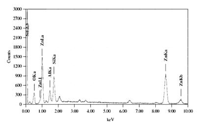
Fig. 7: EDX analysis of 50% ZnO-Bentonite nanocomposite
