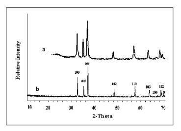
Fig. 2: The XRD pattern (a) prepared ZnO and (b) commercial ZnO
