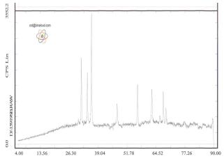
Figure 3 : XRD patern of  $Pb_2(SO_4)O$  produced by calcinations of  $[Pb(bpy)(NCS)_2]_n$
