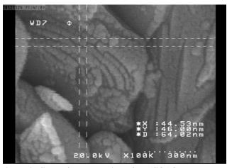
Figure 2 : SEM of nano-particle of Pb<sub>2</sub>(SO<sub>4</sub>)O produced by calcinations of [Pb(bpy)(NCS),]<sub>n</sub>
