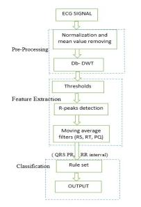
Fig. 1: Block diagram of algorithm
