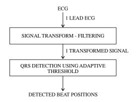
Fig. 2: Pan-Tompkins beat detection algorithm work flow
