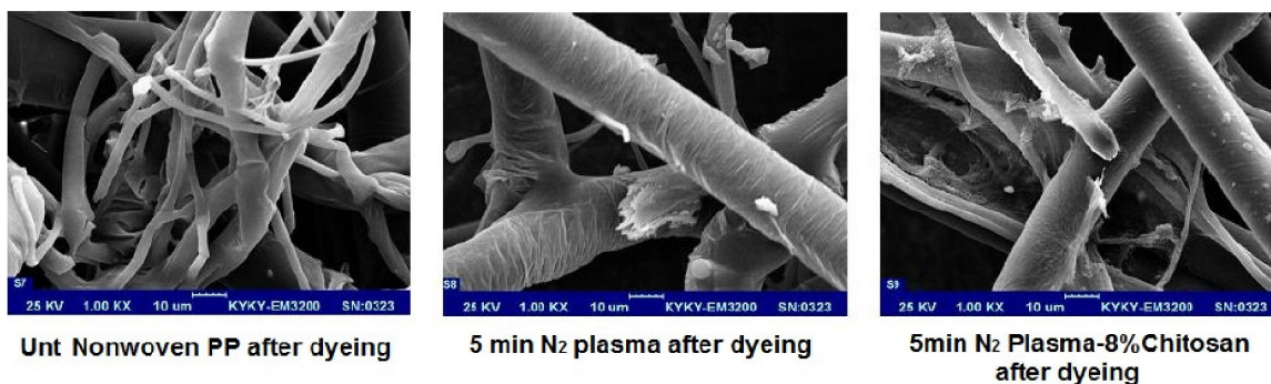
Figure 6 : SEM images of chitosan treated and plasma/chitosan treated PP after dyeing
