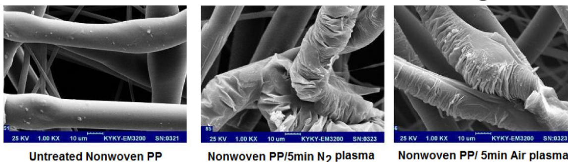
Figure 3 : SEM images of untreated and plasma treated samples
