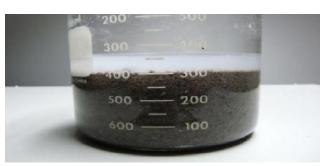
Figure 3 : Fuzzy ball bionic drilling fluid after gel-breaking
