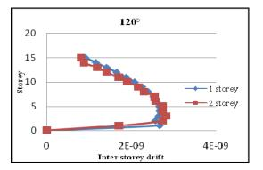
Fig. 10: Interstorey drift profile of 120°
