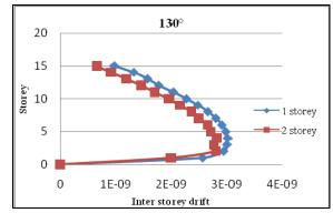
Fig. 11: Interstorey drift profile of 130°
