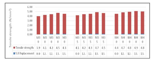
Fig. 4: 28 Days tensile strength (N/mm2)
