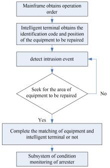
Figure 4: The flow chart of the working process of intelligent monitoring
