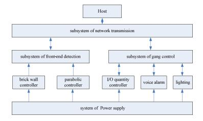
Figure 2: The integration platform block diagram of the background image monitoring system
