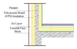
Figure 2 : Thermal insulation of closed roof Division for prevention and treatment of water and soil erosion prevention
