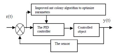
Figure 3: The principle diagram of the control program of improved ant colony algorithm
