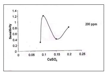
Fig. 3: Variation of sensitivity against CuSO<sub>4</sub>.5H<sub>2</sub>O concentration
