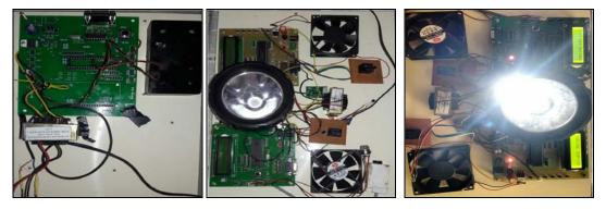
Fig. 4: Receiver, transmitter and output section for Li-fi technology
