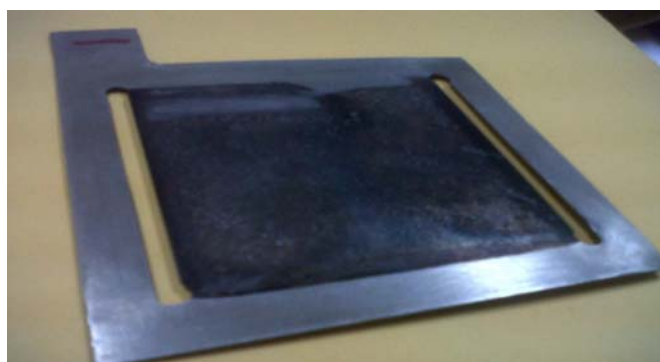
Fig. 12: Corroded titanium electrode
