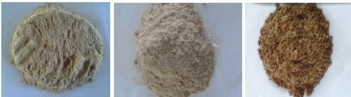
Figure 1: The average particle sizes of saw dust: 0.353mm, 0.767mm, 1.379mm
