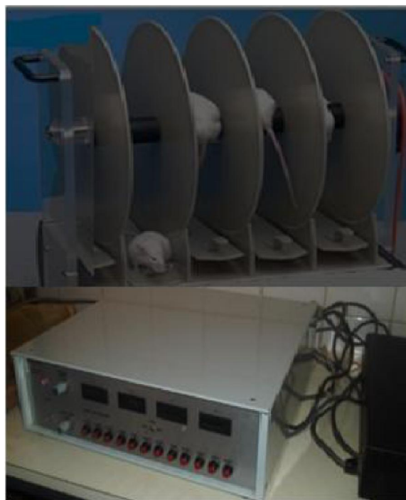
Figure 1 : Rotarod showing three rats walking on the horizontal rotating rod and one falling into its own lane
