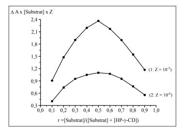
Fig. 2: Job's plot (continuous variation method) of substrates: (1 : ●) and (2 : ■) with HP-γ-CD inclusion complex showing 1 : 1 stoichiometries. Initial concentrations of substrates 1 and 2 are 0.1 mM and 0.01 mM respectively. Absorbance measurements were carried out at 254 nm
