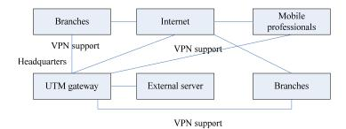
Figure 4 : Network security architecture based on UTM
