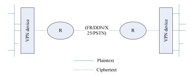
Figure 2 : Schematic diagram of VPN device configuration
