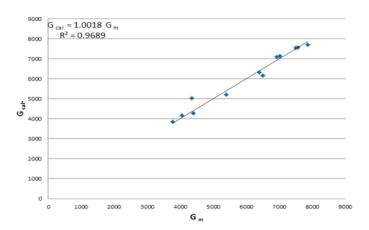
FIG. 2. Comparison between measured (Gm) and calculated (Gc) global solar radiation values for monthly average data through the study period at Qena.
