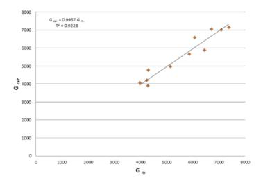
FIG. 1. Comparison between measured (Gm) and calculated (Gc) global solar radiation values for monthly average data through the study period at Mars Matrouh.
