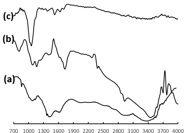
Figure 1: FTIR analysis of hydrogel (a) chitosan, (b) hydrogel C-1 and (c) hydrogel C-4
