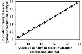
Figure 2: The comparison of assumed and calculated density in direct and reverse hydraulic calculations  $\mu = 45$  c.p
