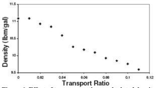
Figure 6: Effect of transport ratio on calculated density for UMP= constant.
