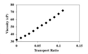
Figure 5: Effect of transport ratio on calculated viscosity for UMP=constant
