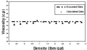
Figure 3: Comparison assumed and calculated viscosity and density in direct and reverse hydraulic calculations for  $\mu$ = 45 c.p
