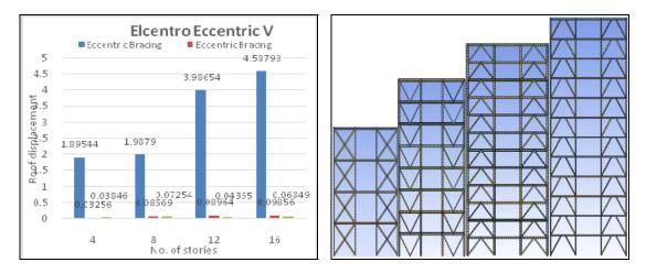
Fig. 2: Comparison in roof displacement of conventional steel braced, SMA braced and the frames with composite arrangement subjected to EI Centro ground motion & Elevation of structures with different bracing patterns
