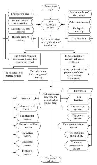
Figure 2 : The early evaluation principle diagram
