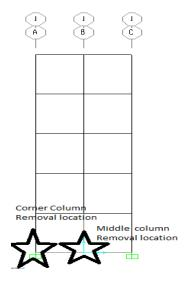
Fig. 3: Diferent column removal location
