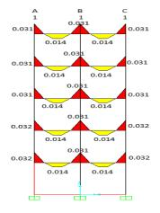
Fig. 5(f): Demand capacity ratio bending moment (DCR) for longitudinal side of fivestory with infill frame building (Corner column removal scenario)
