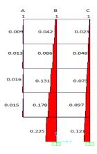
Fig. 5(a): Demand capacity ratio axial (DCR) for longitudinal side of five-story bare frame building (Corner column removal scenario)
