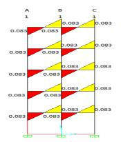
Fig. 5(j): Demand capacity ratio shear force (DCR) for longitudinal side of five-story with infill frame building (Corner column removal scenario)
