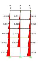
Fig. 5(d): Demand capacity ratio axial (DCR) for longitudinal side of five-story with infill frame building (middle column removal scenario)
