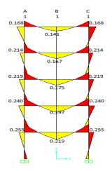
Fig. 5(g): Demand capacity ratio bending moment (DCR) for longitudinal side of fivestory bare frame building (middle column removal scenario)
