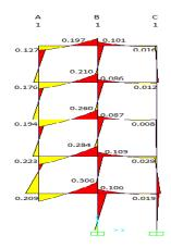
Fig. 5(e): Demand capacity ratio bending moment (DCR) for longitudinal side of fivestory bare frame building (Corner column removal scenario)
