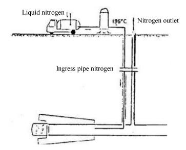
Figure 5 : The diagram of freezing installation
