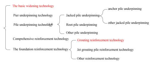
**Figure 2 : Normal foundation reinforcement technologies**
