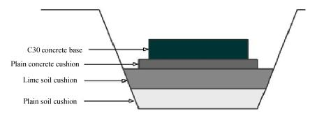
Figure 1 : Diagram of cushion reinforcement technology
