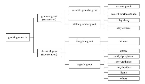
**Figure 3 : The common grouting materials**
