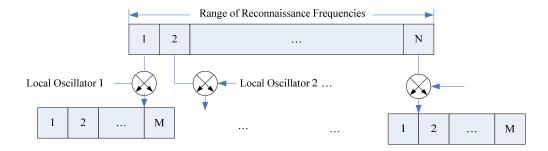
Figure 1 : Schematic diagram of secondary pure channelized receiver
