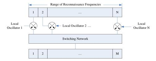
Figure 3 : Schematic diagram of time-division channelized receiver
