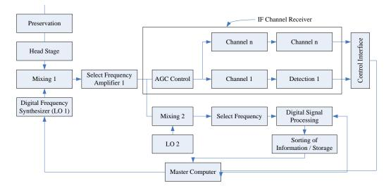
Figure 4 : Composition diagram of composite receiver
