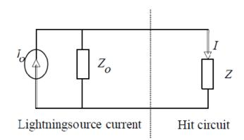
Figure 1: Equivalent circuit of lightning source current
