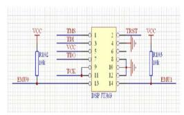
Figure 5: The connection diagram of JTAG
