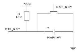
Figure 4: The overall reset circuit
