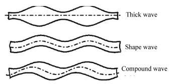
Figure 5 : The geometric characteristics of chattering wave
