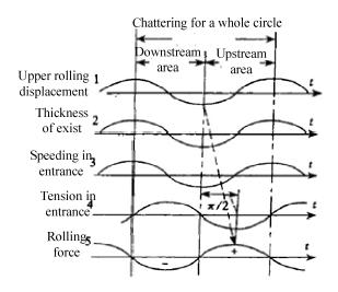
Figure 2 : The forming process of self-exited chattering
