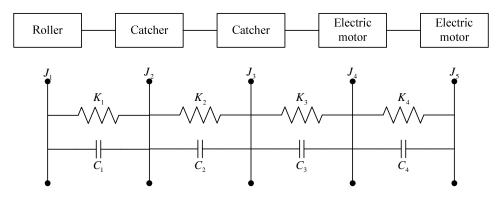
Figure 1: The layout and simplified model of the main drive system of rolling mill
