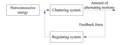
Figure 1 : The constitution of the self-excited chattering system
