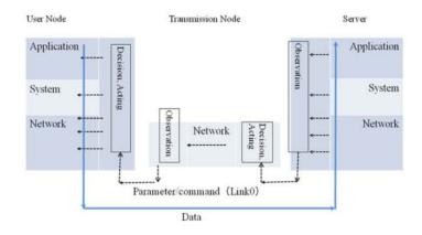
Figure 5 : System architecture
