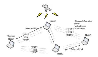
Figure 4 : Wireless network architecture
