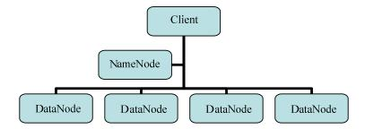
Figure 2: Simplified diagram of hadoop
