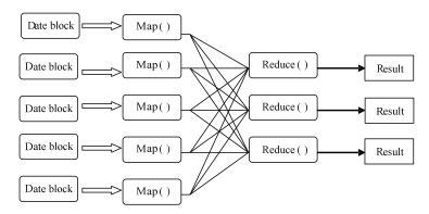
Figure 1: Detailed process of mapreduce
