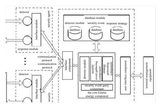
Figure 4: Schematic diagram of enterprise's security management system structure
